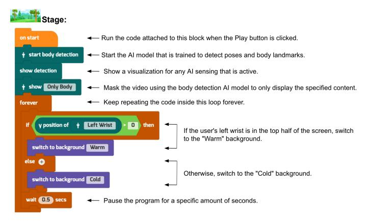
**Note:** This is an open-ended DIY project. Above is an example that uses the provided code blocks to create a Weather Control project.
